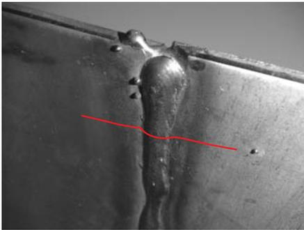
Welding bead / welding seam
