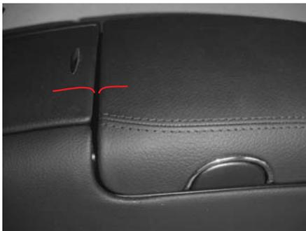
Gap / joining contact
