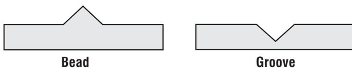
The highest point of a bead has the smallest z-distance value due to scaling from the sensor's viewpoint. The z-distance value is maximum for a groove.
