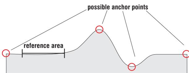
The selection of the anchor point can therefore be adapted to the task in hand. With the scanCONTROL 2810 the following points can be defined as anchor points:
