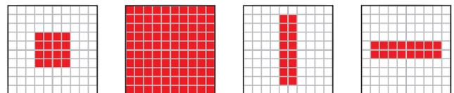
The CMOS array active field (where measurements will be taken) can be programmed according to 96 predefined possibilities, eg. using only a portion of the array increases data acquisition speed, selecting the central area increases accuracy.
