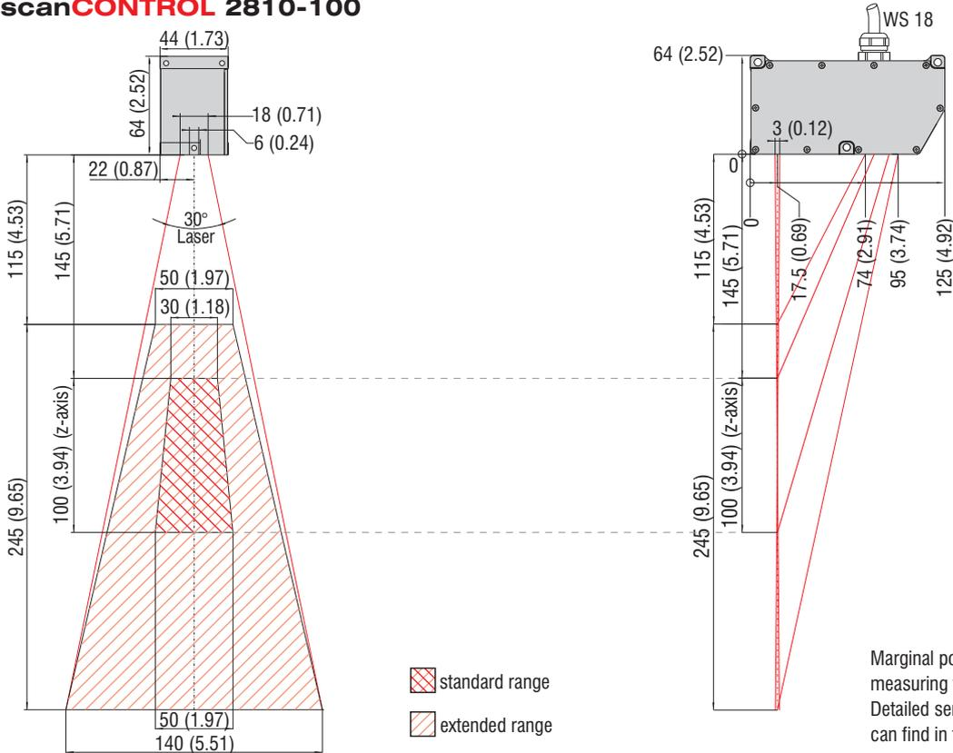
Marginal position tolerance of the measuring field is possible (sensor depending). Detailed sensor and controller dimensions you can find in the scanCONTROL 2800 datasheet.
